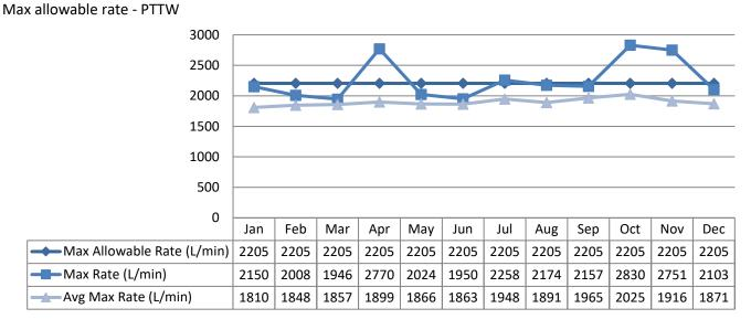
NOTE: Maximum allowable rate was exceeded during brief periods of plant upset when the filter to waste cycle of the backwash sequence needed to be extended to reach compliant turbidity readings.
